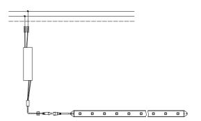
I, One power supply to drive One LED module
